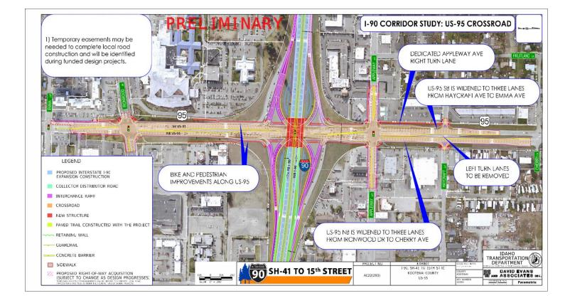
**Scope of Work**. This project will complete the design to replace the existing standard diamond I-90/US-95 Interchange (IC #12) as a Single Point Urban Interchange (SPUI). Work to include widening interchange ramps and extending three lanes in both directions on I-90 from US-95 to 4<sup>th</sup> Street. US-95 will be widened from Emma Ave to Cherry Lane and include bicycle/pedestrian facility improvements.
